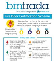
Where the frame and leaf are produced by separate Q-Mark companies, both the frame and leaf must have their own red/green plug.
